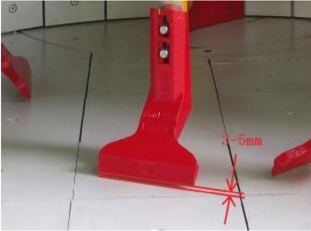
Adjustment Clearance for Mixing Shovel (picture 1)
